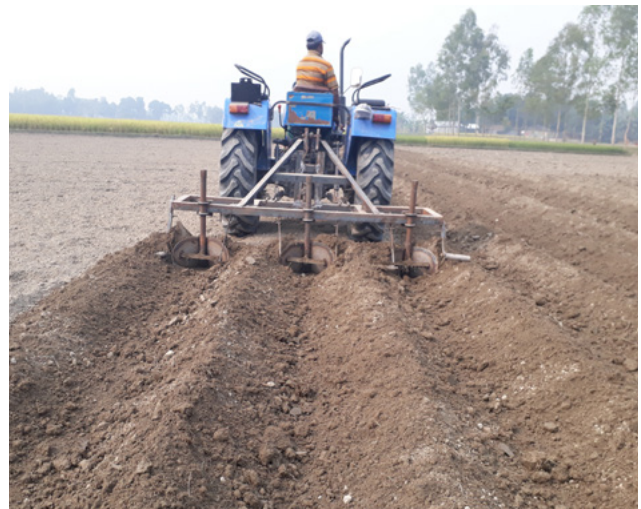
Inter-cultivator to reduce efforts of manual spading
