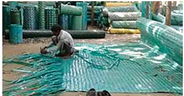
Plastic mats prepared from waste plastic strapping
