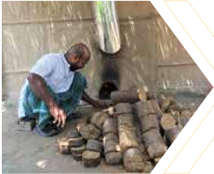
Collected waste briquette prior to curing
